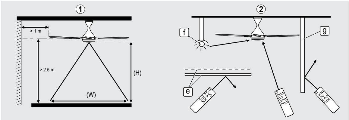
① The figure above shows the best coverage area (W) around 8 m if the height (H) is 4 m. The Remote Control must be pointed to the direction of the Ceiling Fan when in use.
