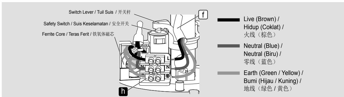
Connect to the power supply according to the wiring instruction below.
