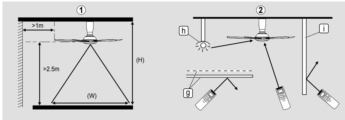
① The figure above shows the best coverage area (**W**) around 8 m. The ideal ceiling height (**H**) is 3 to 4 m. The Remote Control must be pointed to the direction of the Ceiling Fan when in use.
