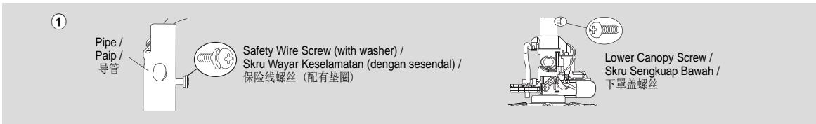
② Pull down Lower Canopy until it stop and fix to Pipe firmly by screwing them as shown.
