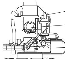
1. Pastikan Tuil Suis menekan Suis Keselamatan. / Make sure Switch Lever press the Safety Switch. / 确定开关杆按压保险开关。
