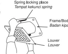
Attach the louver to the frame/body by fixing the spring into the spring locking place.
