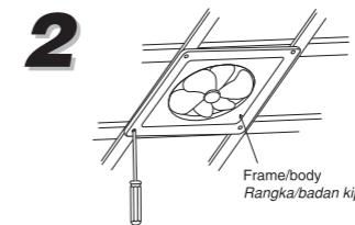
Install the set to the wooden frame using the screws.
