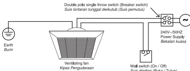
This product is not provided with plug or with other means for disconnection from the supply. When connect or change the power cord or lead wire, it must be replaced by the qualified persons in order to avoid a hazard. Please use 227IEC53(RVV) or thickness of tube is 1mm or above. (Other requirements such as diameter of lead wire, please done according to the regulation of the country).
