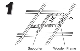
Fix wooden frame to ceiling where the set is to be installed.
