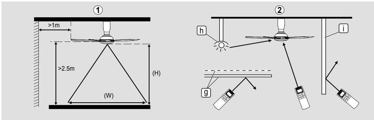
① The figure above shows the best coverage area (W) around 8 m if the height (H) is 4 m. The Remote Control must be pointed to the direction of the Ceiling Fan when in use.
