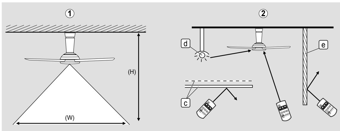
① The figure above shows the best coverage area ( $W$ ) around 8 m. The ideal ceiling height ( $H$ ) is 3 to 4 m. The Remote Control must be pointed to the direction of the Ceiling Fan when in use.
