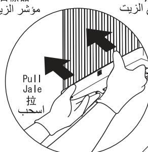
Hold knobs and pull the oil cup like picture.
